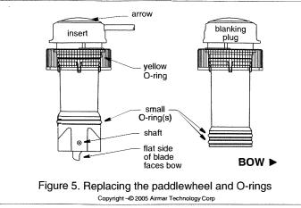
weeks. Clean the insert with a Scotch-Brite® scour pad and mild household detergent, being careful to avoid scratching the depth transducer. If fouling is severe, remove the paddlewheel (see step #1 below). Lightly wet sand it with fine grade wet/dry paper.
