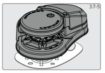
5. Place the base mat in position on the deck. Optionally, apply a suitable sealant to the base of the windlass, any mounting pad or around the studs. NOTE: If using silicone or other rubbery type sealant, it is advisable to allow curing of the sealant before final tightening of the mounting nuts.
