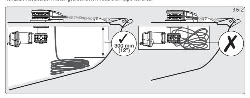
2. There must be sufficient vertical fall for the chain or rope when hauling in.
