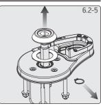
Assemble the new gypsy in reverse order, note that the part number engraved on the stripper ring should face upwards.
