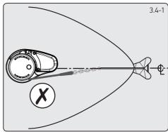
If a pad is required for these models, care must be taken to ensure that the windlass base is parallel to the motor/gearbox mounting flange. Shims may be used, before the motor/gearbox is installed, to correct minor misalignment.
