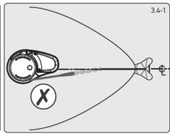
2. If a pad is required for these models, care must be taken to ensure that the windlass base is parallel to the motor/gearbox mounting flange. Shims may be used, before the motor/gearbox is installed, to correct minor misalignment.
