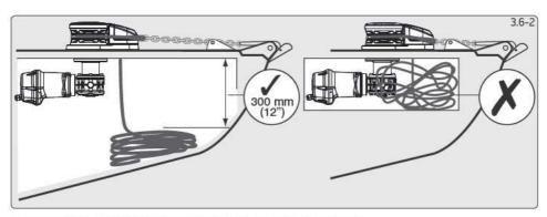
2. There must be sufficient vertical fall for the chain or rope when hauling in.
