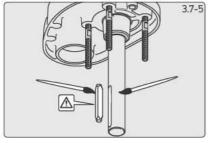
Lightly coat the shaft with grease and ensure the drive key is in place before assembly to motor/gearbox.
