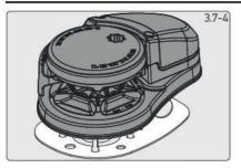
4. Place the base mat in position on the deck. Optionally, apply a suitable sealant to the base of the windlass, any mounting pad or around the studs. NOTE: If using silicone or other rubbery type sealant, it is advisable to allow curing of the sealant before final tightening of the mounting nuts.
