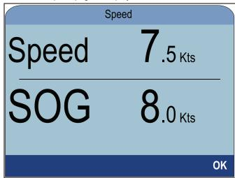
The Check Speed page can also be accessed from the Edit calibration options menu: Advanced > Adjust cal table > Start > Options > Check speed.
