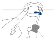
Attach the sensor by twisting clockwise until it clicks. If the battery is missing or inserted incorrectly, it will be impossible to click the alarm in the mounting base.
