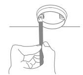
3. Use enclosed screws and plugs to install the mounting base on the marked position.
