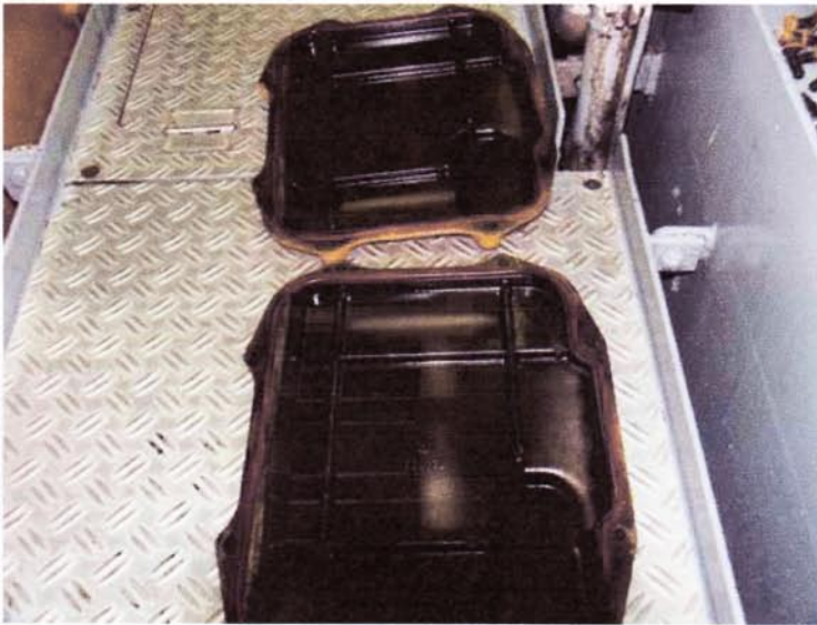
Visual inspection of soot deposits on the crankcase cover
