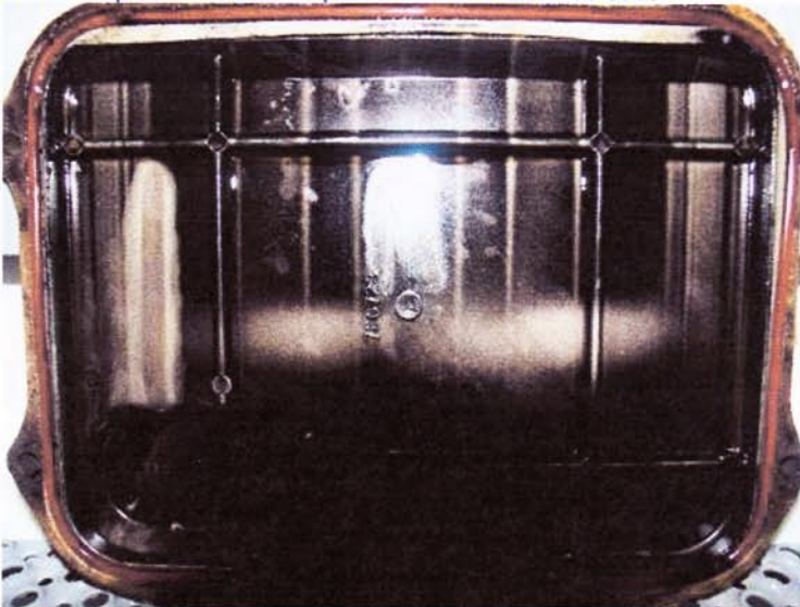
Visual inspection of soot deposits on the crankcase cover
