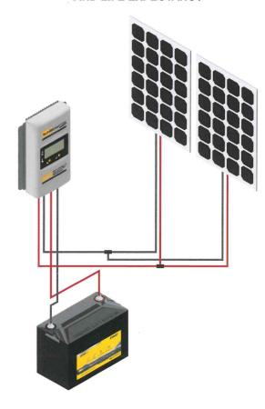
FOR 24V & 48V SYSTEMS IT IS COMMON TO PUT THE SOLAR PANELS IN SERIES BUT WE RECOMMEND THE USE OF A "BOOST" CHARGE CONTROLLER WHICH ALLOWS A PARALLEL INSTALLATION
