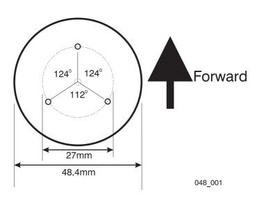
Mounting: Drill 3 x Holes (size depends on the material being drilled)
